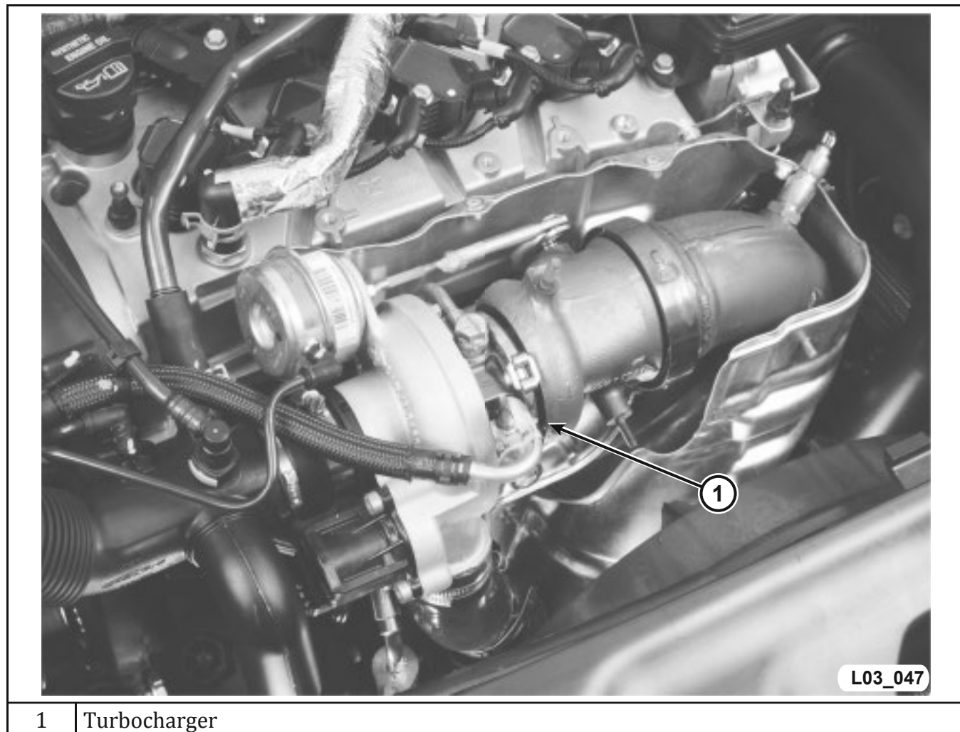
Figure 119 Typical Turbocharger
