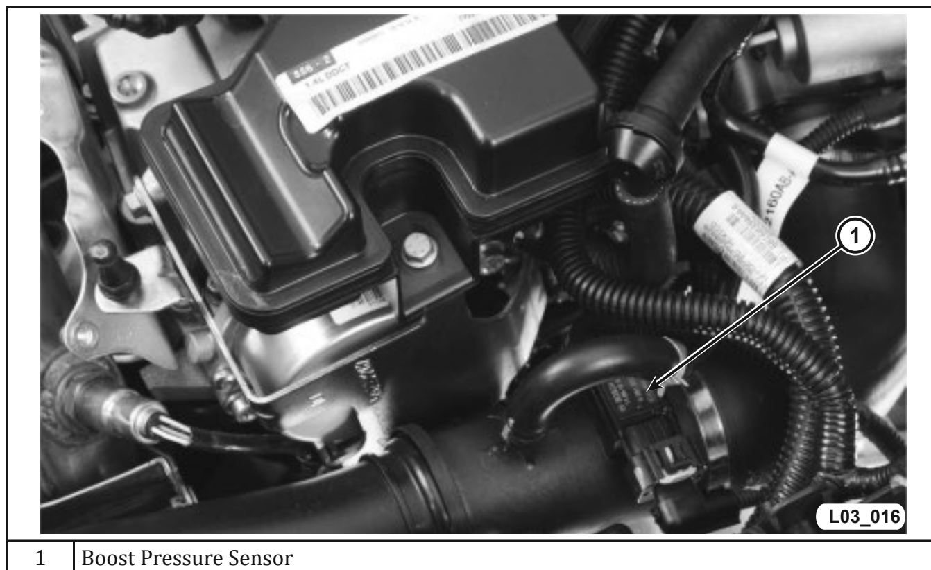
Figure 121 Boost Pressure Sensor
