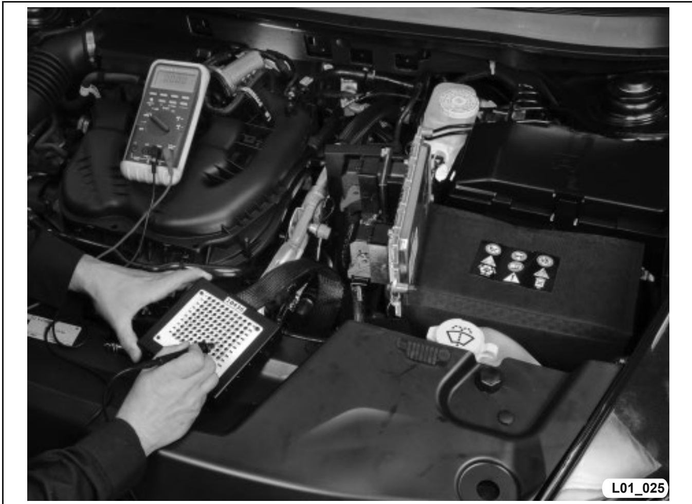
Figure 16 Voltage Drop Across Ground Terminal - DMM Set to DC Volts
