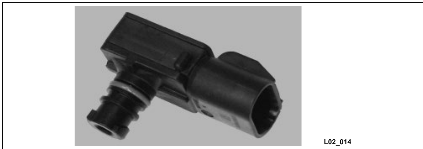
Figure 30 Typical MAP Sensor
