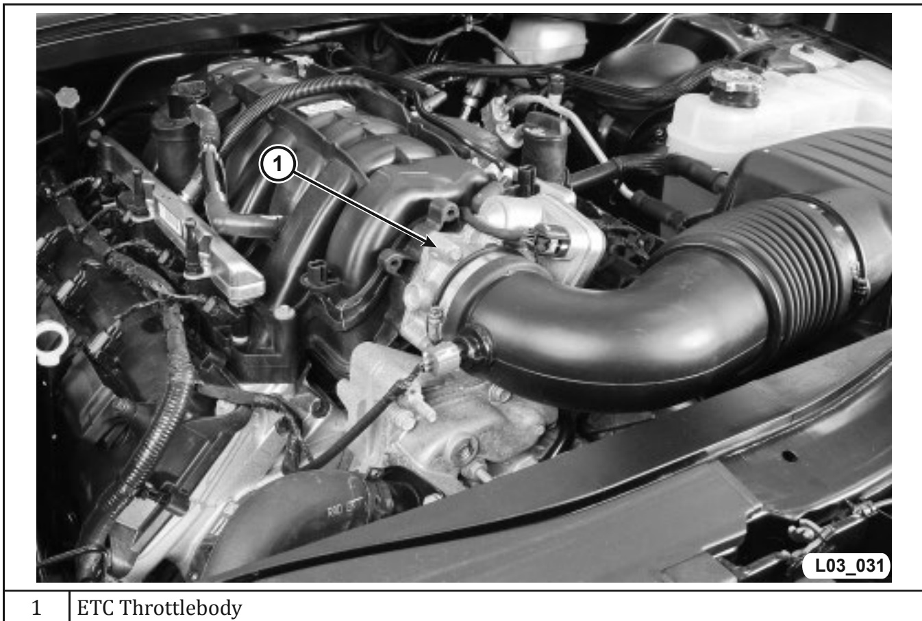
Figure 83 ETC Throttlebody
